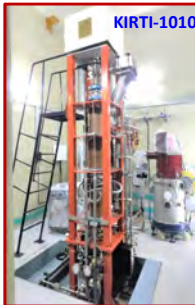
10 MeV, 10 kW Linac deployed at M/s MSSPL Bangalore
